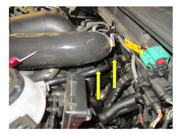
7. Next you will need to separate the breather hose. To do this you will need a heat gun or hair dryer. Give the hose some heat for about 30 seconds or so, then pull the hose away from the joiner.
