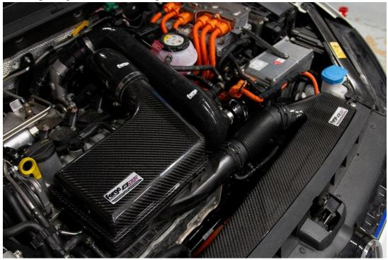
**15.** Fit the carbon fibre enlarged front duct into position using the 2x M6 fasteners provided. When fitting the carbon duct you will have to move the orange power cable, simply remove it from its retaining clip and move the cable backwards.
