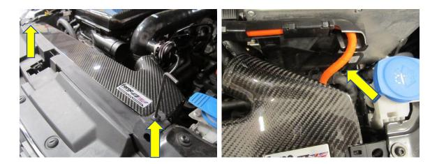
**16.** <u>Fit the OEM flexi pipe from the carbon duct to the carbon airbox.</u>
