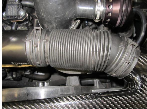
**17.** Tighten the hose clamps on the turbo inlet pipe, being cautious not to over tighten the hose clamp on the carbon fibre lid as this could crack and fracture if over tightened.
